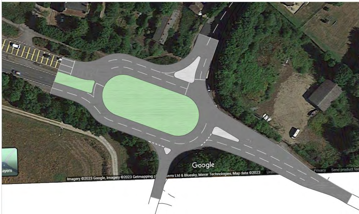
Figure 8-4 – Kippings Cross Partial Signalised Roundabout Junction
